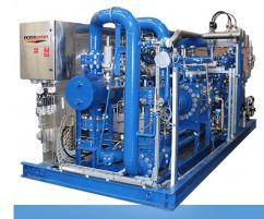
A 250kW Anax-Star prototype Turboexpander (ASTE) was field evaluated by GTI at the DNV GL Flow Centre in the UK, and was found to overcome obstacles that have prevented widespread adoption of GLGs.
