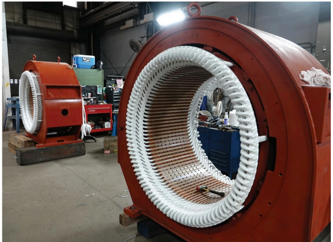
Two large motors after a rewind and refurbishment at Longo’s Wharton facility.
