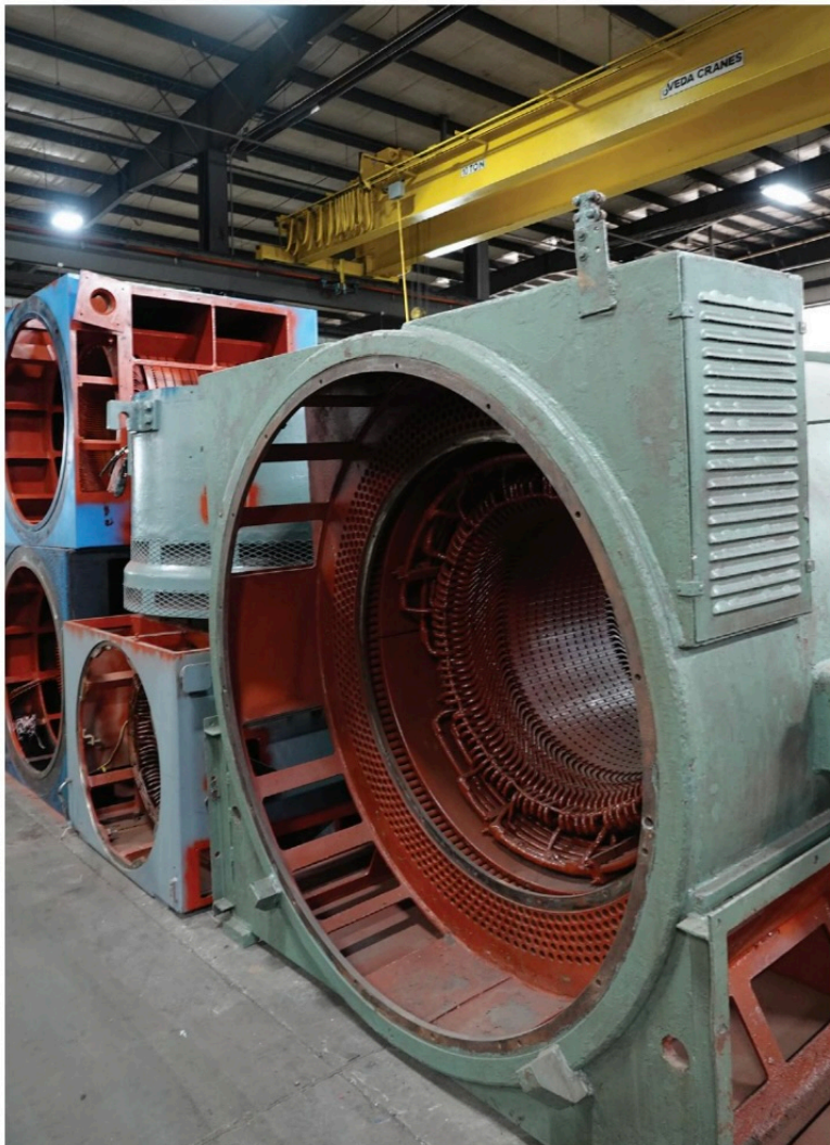
Longo’s Wharton facility provides in-shop maintenance and repair services on up to 15,000 hp motors (rewind/redesign), 30 MW hydrogenerators, and 100 MW turbogenerators.
